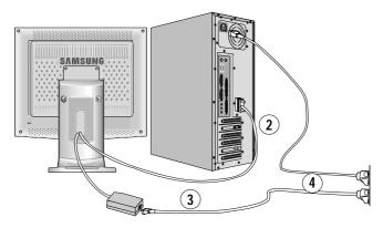
Figure 3. Cable connections (Analog)
